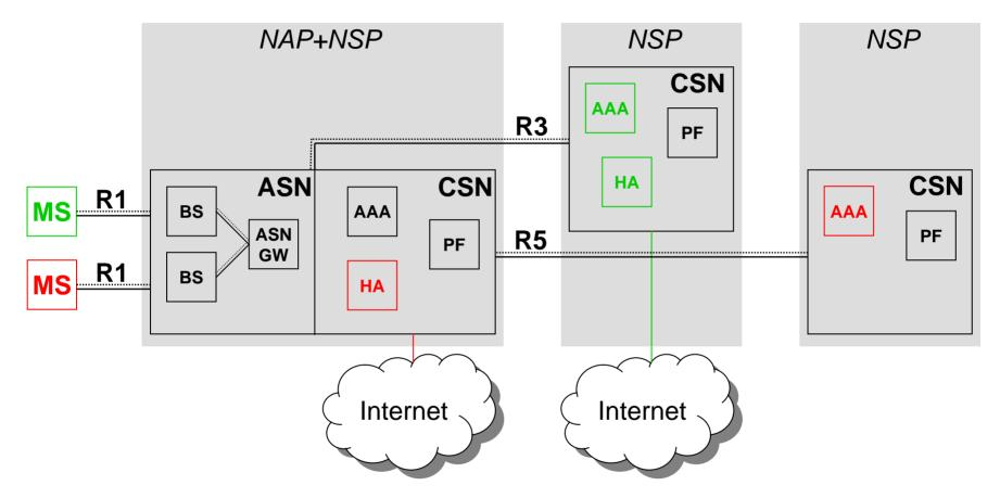
Most access provider will implement direct Internet connectivity by a co-located CSN to minimize transport costs.
