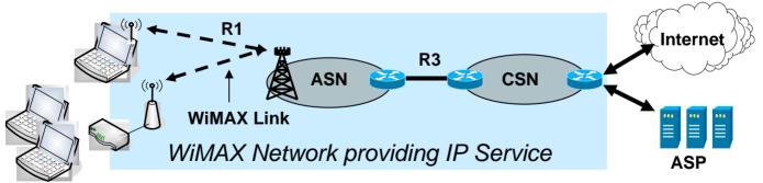
The WiMAX network provides IP connectivity to the Internet and operator services for single hosts or multiple hosts behind a gateway.
