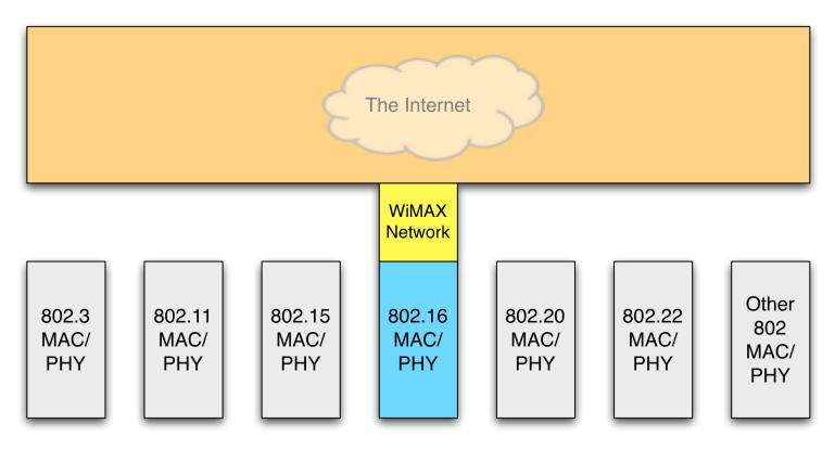
WiMAX Network provides operator-required services to 802.16 devices: authentication, provisioning, mobility management, QoS management, roaming...
