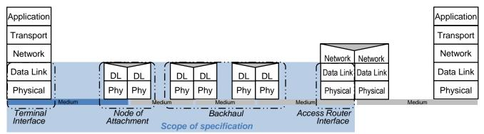
• IEEE 802 access network describes the layer 2 network between terminal and access router implemented through IEEE 802 technologies.
