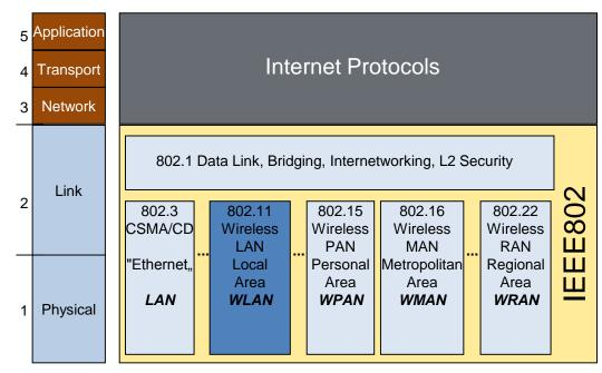
Specifies only Physical and Link Layer. Complete set of standards for carrying IP
